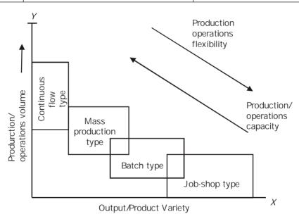
Fig. 1.4: Production and operations system.
